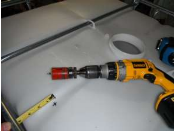
Mark 4" from inside rail centered from front to back...
